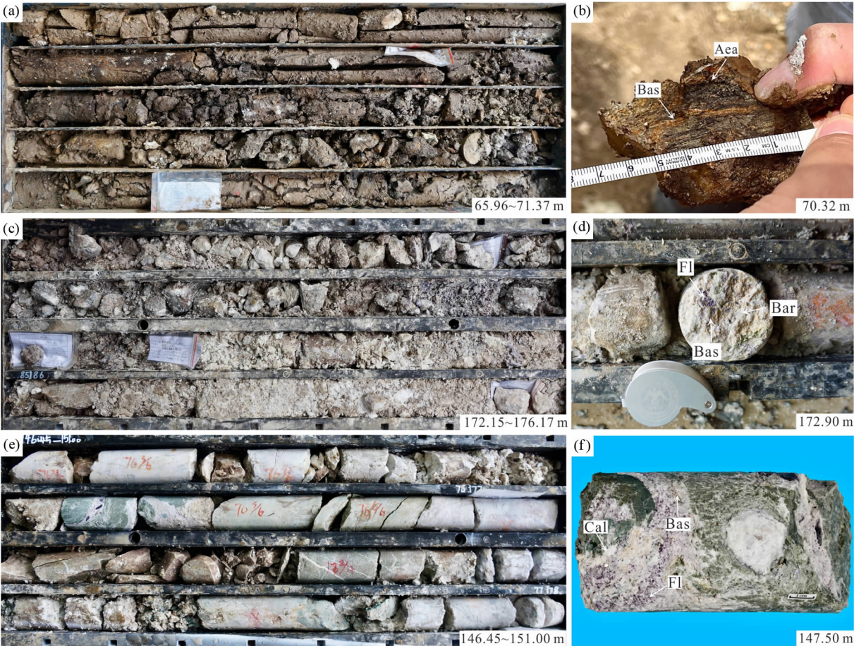
图5 龙家沟地区 ZK001 钻孔矿石特征 (a) 风化灰黑色霓辉石型脉状矿石; (b) 条带状霓辉石型脉状矿石; (c) 灰白色方解石型脉状矿石; (d) 方解石型脉状矿石; (e) 角砾状矿石; (f) 角砾状矿石手标本特征。Aea-霓辉石; Bar-重晶石; Bas-氟碳铈矿; Cal-方解石; Fl-萤石 Fig. 5 Ore characteristics in ZK001 from Longjiagou area (a) weathered gray-black aegirine-augite type vein ore; (b) strip aegirine-augite type vein ore; (c) gray-white calcite vein-type ore; (d) calcite-type vein ore; (e) characteristics of breccia ore; (f) characteristics of hand specimens for breccia ore. Aea-aegirine-augite; Bar-barite; Bas-bastnaesite; Cal-calcite; Fl-fluorite
